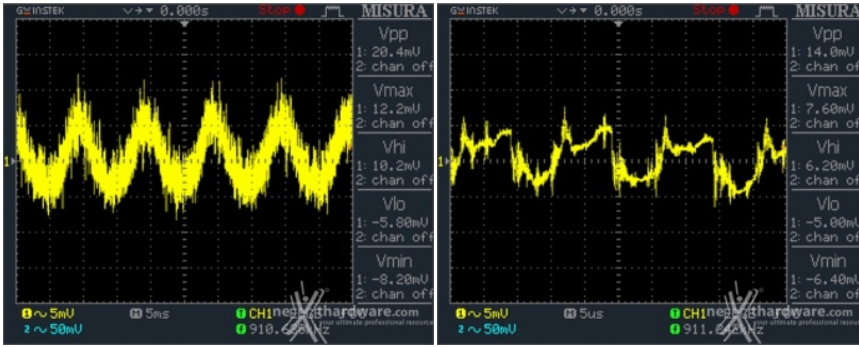
Low Frequency Ripple 12V @ 50%
