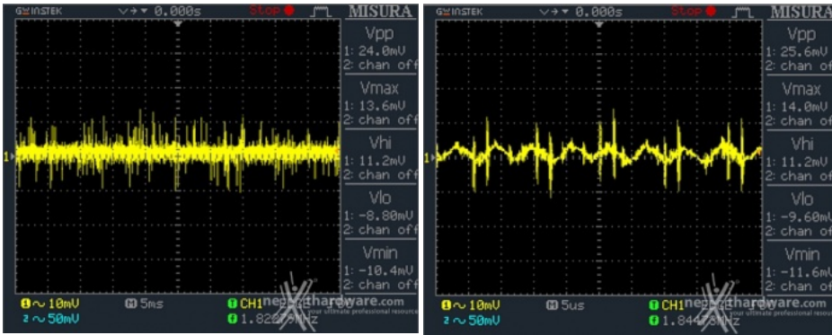
Low Frequency Ripple 5V @ 0%
