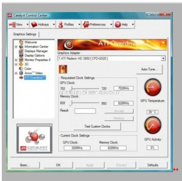
VGA Idle, GPU 300 Mhz, Temp. 39↔°
