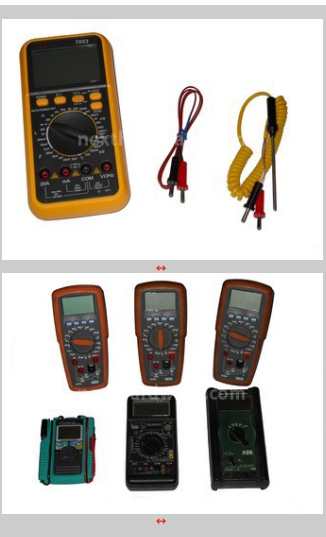
Multimetri: 3 x HT81 1 x ABB Metrawatt M2004 1 x Edes ELD9102 1 x Kyoritsu Kew Model 2001 1 x EDI T053
