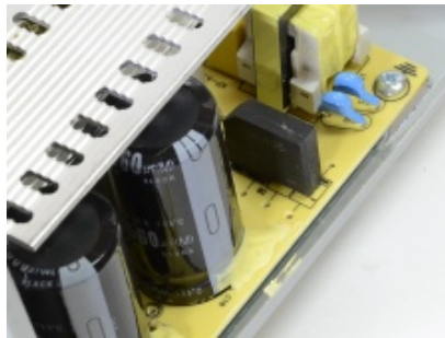
Ponte raddrizzatore KBL406 ( http://dalincom.ru/datasheet/KBL406.pdf )
