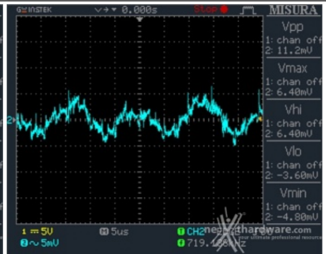
PWM Frequency Ripple 5V @ 50%
